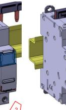
Pull the device downward in order to release it completely from the prongs of the busbar
