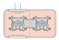
IP55 sealing on front part (cover) on the box is ensured by rotating four 1/4 turn fixings.
